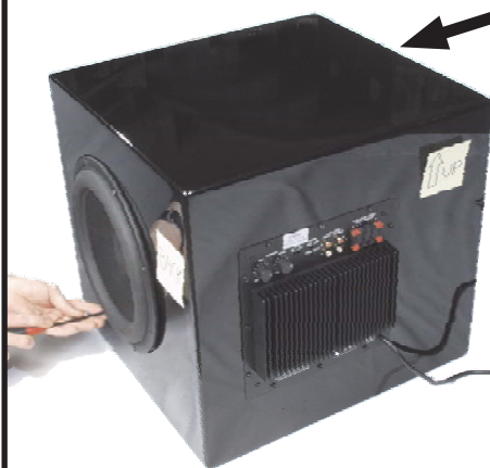
APPLYING GASKET TAPE AROUND THE DRIVERS IS VERY IMPORTANT !
