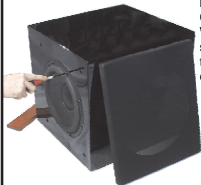
APPLYING GASKET TAPE AROUND THE DRIVERS IS VERY IMPORTANT !
