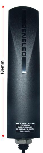
The ANT516 is an economically priced, compact, unity gain 5G antenna suited for use in the bands 690-960, 1710-2700 & 3575-3700 MHz. It comes standard with 3 metres of low loss cable terminating in an SMA male connector & is suited for mounting onto a wall bracket.
