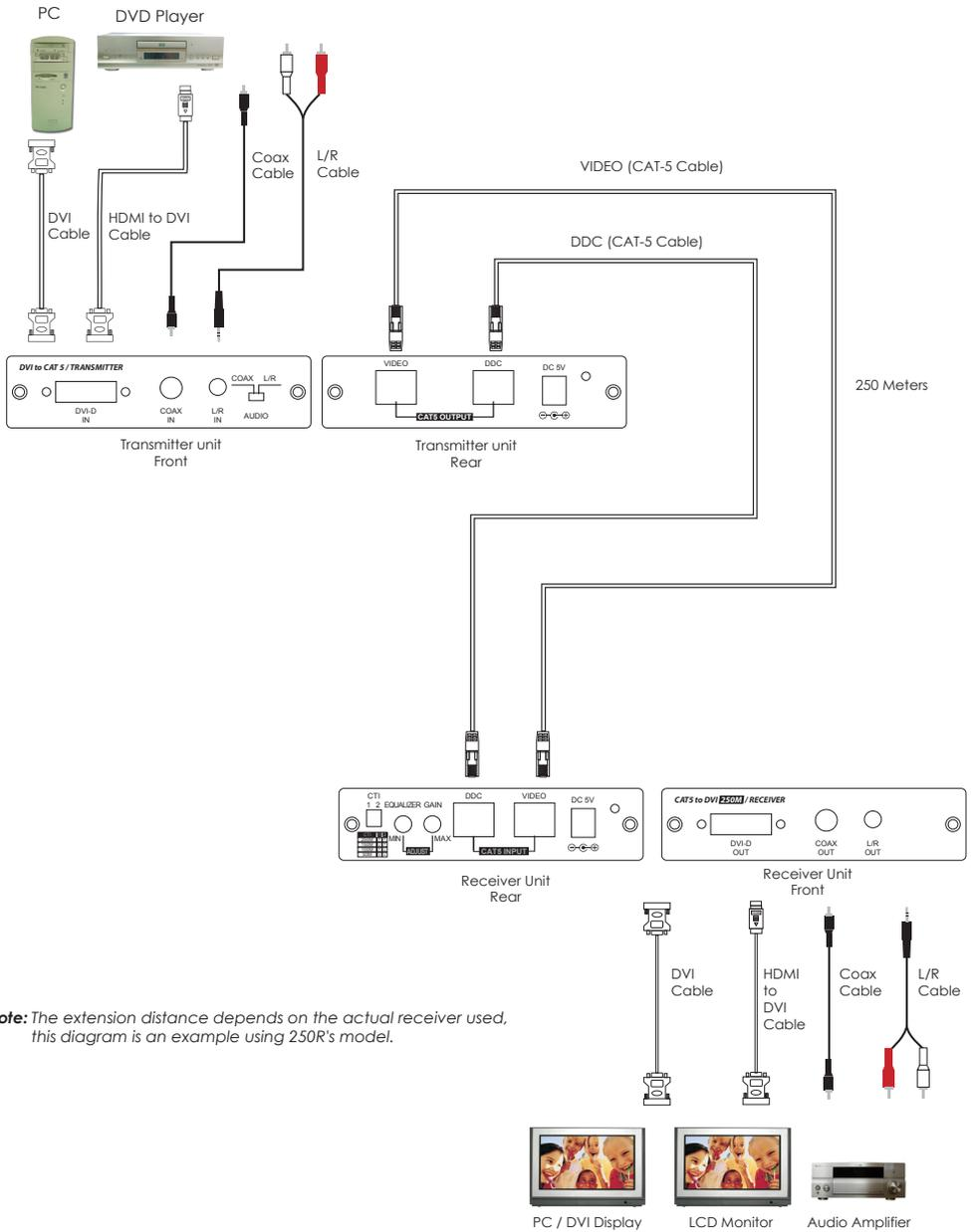
**Note:** The extension distance depends on the actual receiver used, this diagram is an example using 250R's model.
