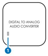
1 POWER LED: The LED will illuminate in red when the power is connected.
