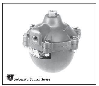
The driver voice coil impedance shall be eight ohms. The internal driver will employ a linen-based, molded phenolic diaphragm, 1½-inch diameter voice coil and "rim-centered" ferrite magnet structure. Replacement part 353 voice coil and diaphragm assembly shall be available.
