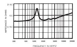
Figure 3. Impedance Response - Plane Wave Tube (1 inch)
