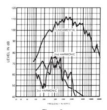
Figure 3 850T Frequency Response (1 watt at 1 meter)
