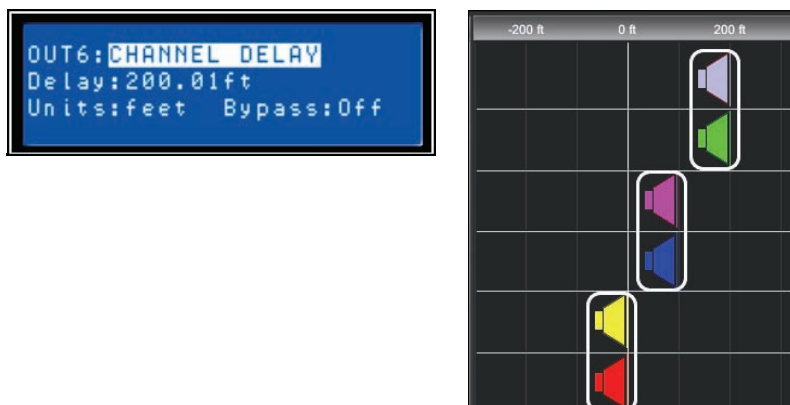
Illustration 5.3: Here Output 5 and 6 are linked and their delay is set to 200 feet. Output 3 and 4 are also linked and set to 100 feet. In this configuration, speaker outputs 5 and 6 are said to be 200 feet in front of Main speaker output array 1 and 2. The effect of air temperature on the actual delay time will also be automatically calculated based on the Temperature Parameter in the Setup Menu. See Output Linking.
