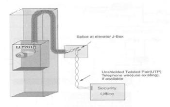
\* Video signal transmitting through video balun transceiver in elevator will efficiently decrease interference.
