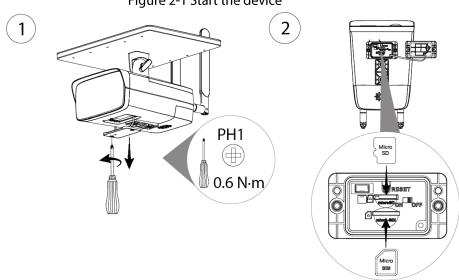
Figure 2-1 Start the device
