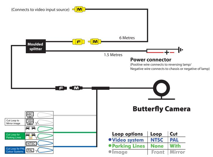
**Note:** When cutting loop wire make sure unit is turned off
