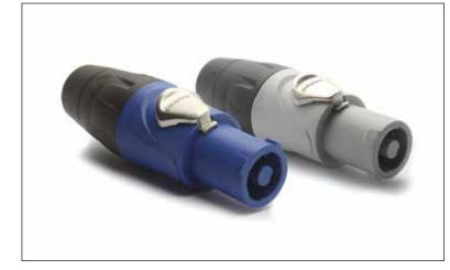
HP Series connectors are suitable for AC power supply where a latch locking connector is required. They are rated at 25 A / 250 Vac. Connectors are keyed and colour coded for power-in (Blue) and power-out (Grey).
