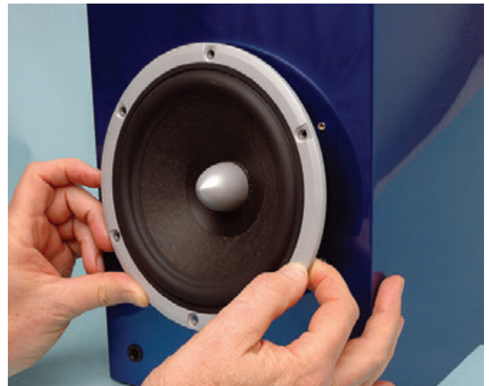
Fit the woofer carefully and do not touch the cone at this point, otherwise you may damage it. It is secured to the baffle with six Allen screws.
