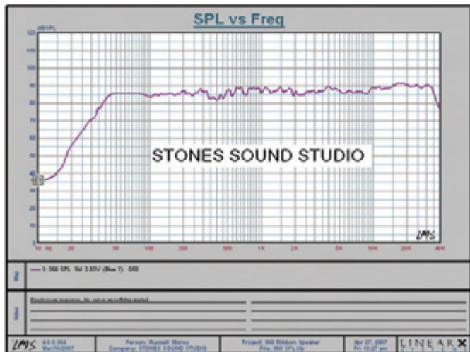
The overall frequency response of the Signature Series HD260 and HD360 speakers is commendably flat to below 50Hz. This is the response of the HD260.
