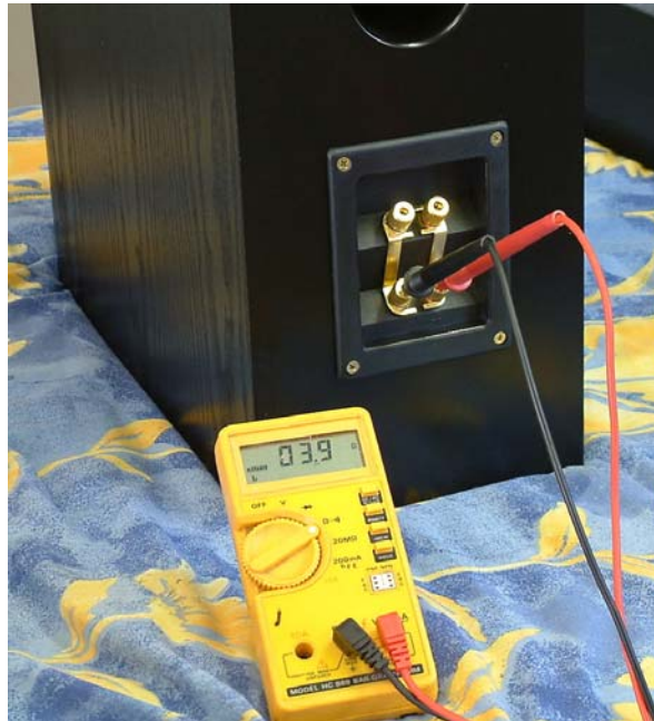
Photo 3 DMM ohm measurement of the 260-260C speaker Crossover Network Resistance (dc only)
