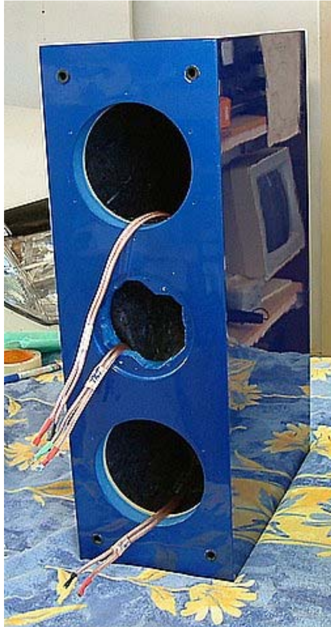
Speaker push on connector cables fitted through front speaker mounting whole cutouts
