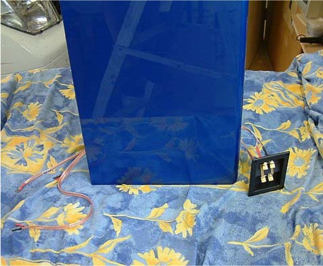
Fit speaker 4 terminal cup through felt and rear panel mounting hole then secure with 4 MDF countersunk wood screw
