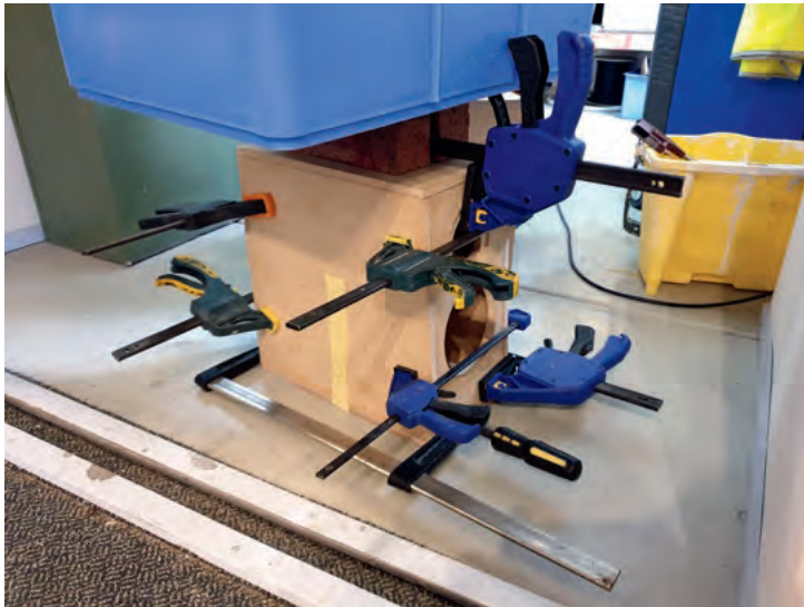
Photo 4: one Active Monitor speaker box, glued and clamped, waiting to dry. This sat for 24 hours before further work was undertaken.
