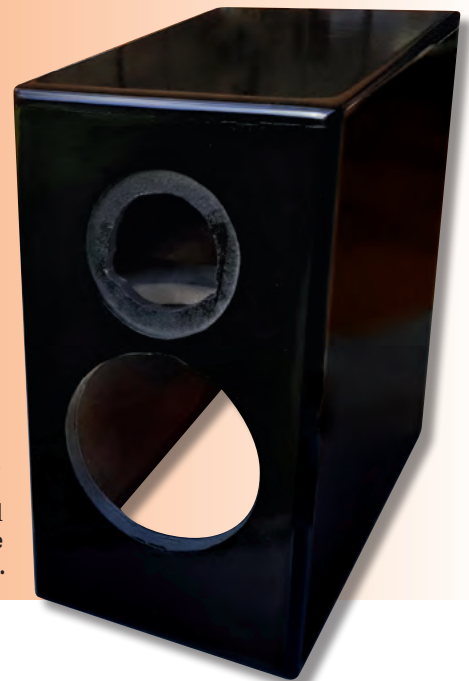
Photo 5: the primed Active Monitor speakers drying in front of the air conditioner. These were later sanded smooth before applying spray primer, then sanded again before the top coat.
