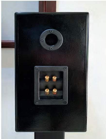
Photo 7: the rear of the speaker, showing the texture you get if you don't sand the undercoat. This also gives you a good view of the vent and the terminals.
