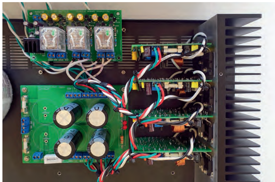
Photo 13: the wiring to the Speaker Protector is easier to do before you have fully mounted it in the chassis. Note the removal of the rear panel to gain some extra space while doing this.
