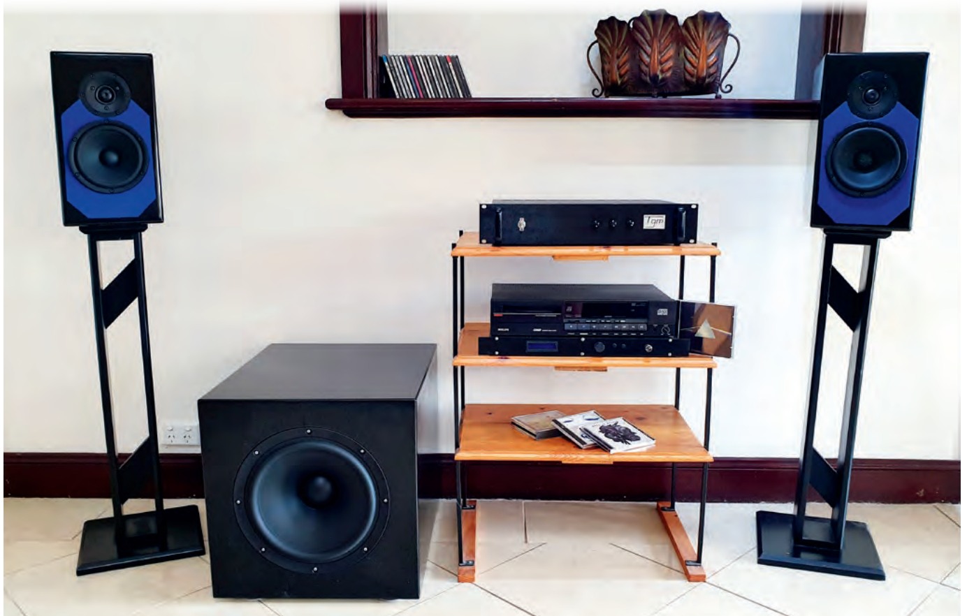
The finished speakers shown with subwoofer and Philips CD player. The speakers can be mounted on top of 800mm tall stands, as shown here, bringing them to about ear height when seated (see the parts list).
