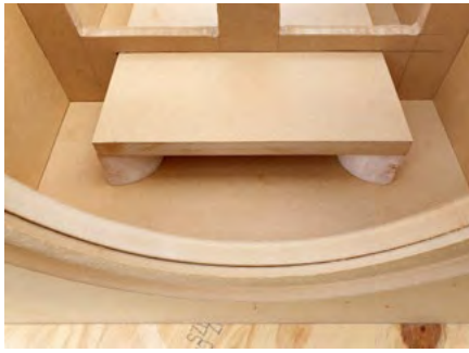
Photo 2: My home-made circle jig allowed me to create a clean circular rebate and cut out the driver hole perfectly.
