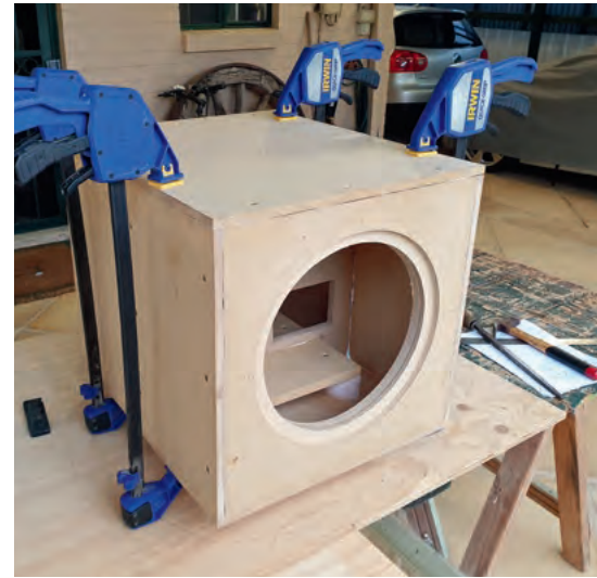
Photo 8: after installing the top panel, I applied clamps liberally and waited for it to dry. You can see the exit of the port and the flush fit of the brace to the top panel of the port here.
