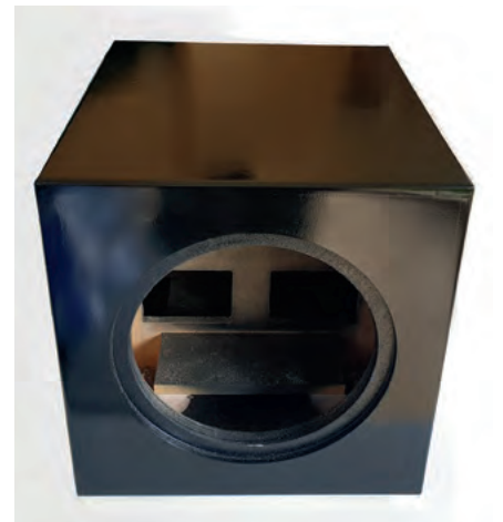
Photo 10: the Active Subwoofer with the final coat of "rattle can" black paint. It's supposed to be satin but looks a lot like gloss.
