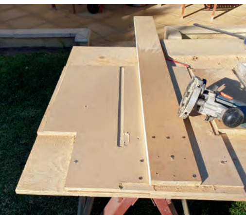
Photo 1: with a router and some MDF off-cuts, you can build a jig to make precisely aligned rebates.
