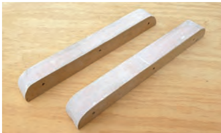
Photo 3: the stack of panels after the rebates and holes have been made. The vent sides are on the top of the pile (and shown below). They are made from three layers of stacked MDF glued together & sanded smooth.
