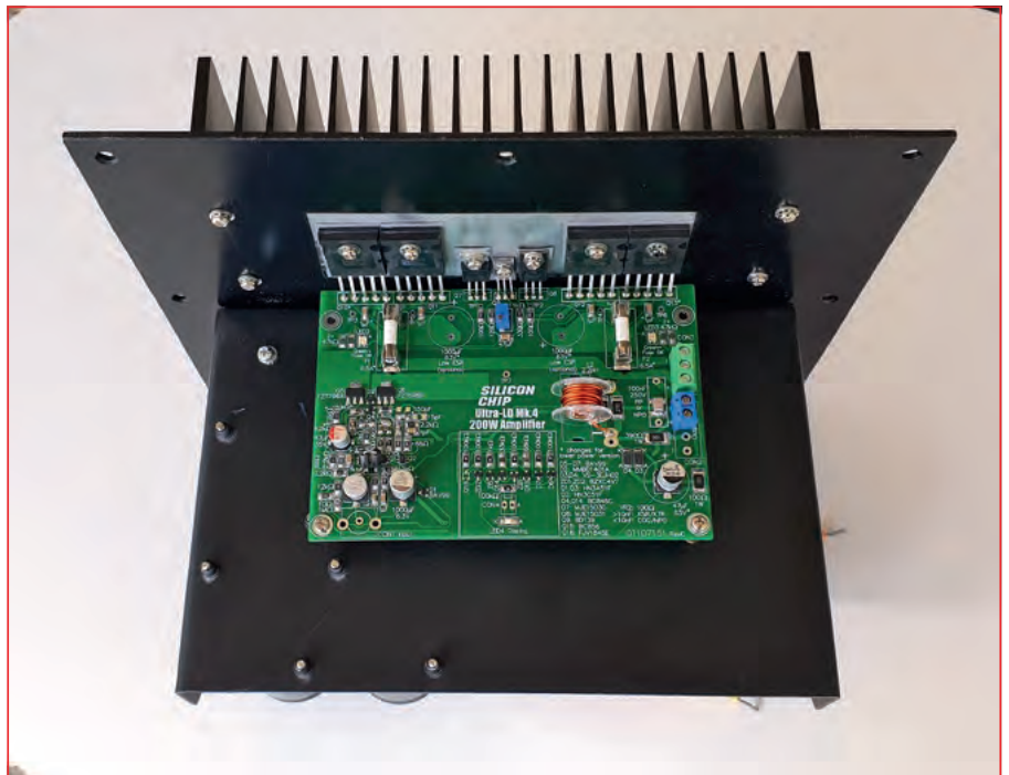
Photo 12: The Ultra-LD Mk.4 amplifier attached to the bracket, ready to be wired up.
