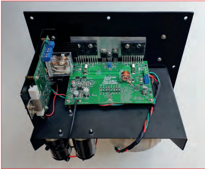
Photo 15: this is how the amplifier side of the module looks after construction and wiring is complete.
