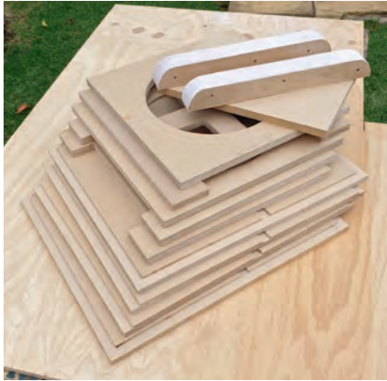
Photo 3: the stack of panels after the rebates and holes have been made. The vent sides are on the top of the pile (and shown below). They are made from three layers of stacked MDF glued together & sanded smooth.
