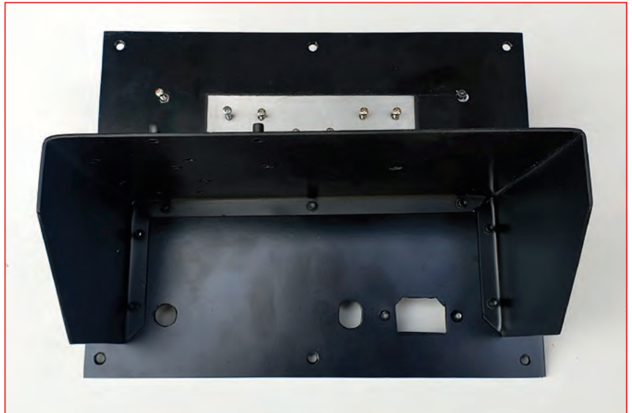
Photo 11: The majority of the plate amplifier parts mount on this bracket.
