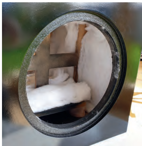
Photo 16: I used a staple gun to attach a double layer of poly wadding I bought at Lincraft. This is required to dampen rear emissions from the driver and reduce resonances.
