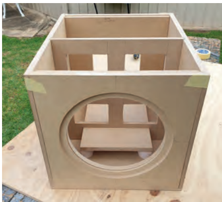
Photo 5: it's critical to 'dry fit' everything together before applying glue. If you start gluing and find a problem, it will be harder to fix.
