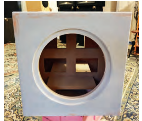
Photo 9: I sanded and primed the active Subwoofer, then sanded it again and added a few filler touch-ups to make the joins perfectly smooth.
