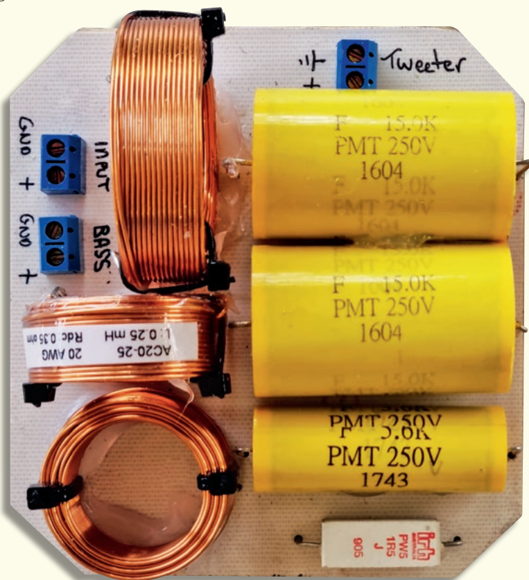
The prototype crossover was simple enough that we made the PCB ourselves. We recommend using electrolytic crossover capacitors instead of the two large 15µF polypropylene capacitors shown here.
