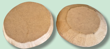
Photo 2: we roughly cut two 120mm MDF discs from off-cuts (left), then used an 80-grit sanding disc in a cordless drill chuck to shape it to fit in the bottom of the bowl (right).
