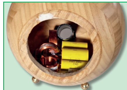
Photo 7: this close-up shows how the crossover board is orientated so the closest inductor just misses the port tube.
