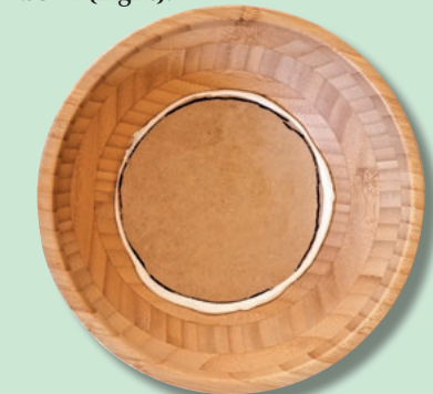
Photo 3: the reinforcement disc is glued into the bottom of the bowl using acrylic gap filler. Before doing this, ensure it is a close fit, leaving gaps less than 5mm wide all around.
