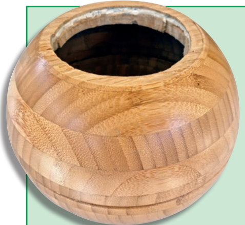
Photo 4: the result of cutting a 102mm diameter hole in both the base of the bowl (already routed to have a larger flat area) and the MDF reinforcement disc, leaving just a ring.
