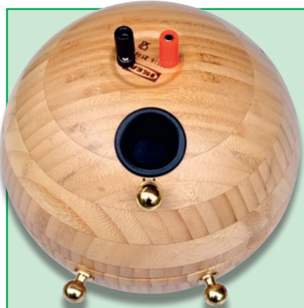
Photo 5: the flat part of the base opposite the driver cutout provides a place to mount the two binding posts, while the port is offset so it fires downwards and clears the internal crossover assembly.
