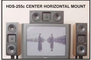
Big sound from a compact box. Fully Shielded for TV Home Theater. Impressive Hi-Fi System Upgrade Excellent for matching with our 8" or 12" Subwoofer Systems. Speaker Stand or shelf mounted. Rear vented. Tapered internal edges. Time corrected, counter-sunk tweeter. Coaxial MTM design. Curved grills. Frequency 42Hz to 22KHz H495 x W180 x D305mm Power Amp 10 to 100 Watt 80hm nominal Sensitivity 92db
