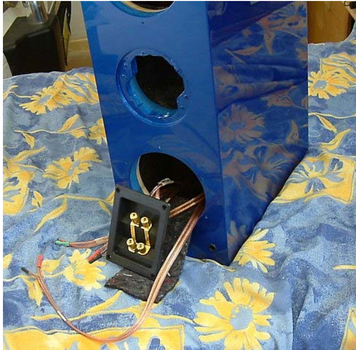
Fit crossover assembly through lower woofer hole and secure with six Velcro tabs
