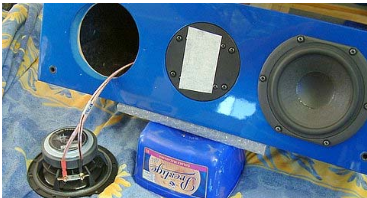
260 C CENTRE showing peerless bass/mid connections
