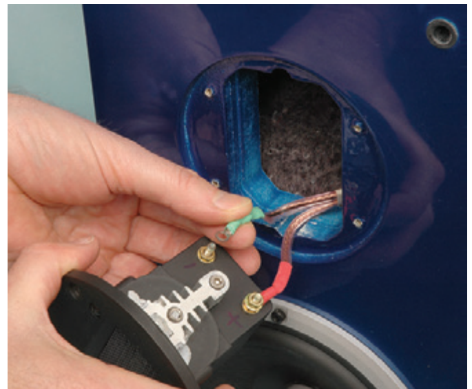
Making the connections to the tweeter. Do it exactly as the photo depicts. Don't over-tighten the nuts on the tweeters – it would be a shame to damage such a magnificent performer.
