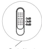
Tweeter Attenuator Adjust to desired sound
