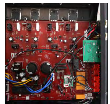
Built-in digital to analogue converter with digital signals up to 24bits/96Hz
