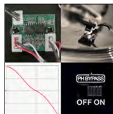
RIAA Phono pre-amplifier to support turntable input
