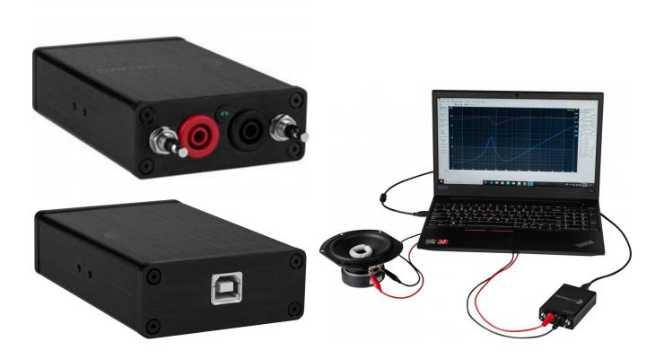
DATS V3 Computer Based Audio Component Test System
