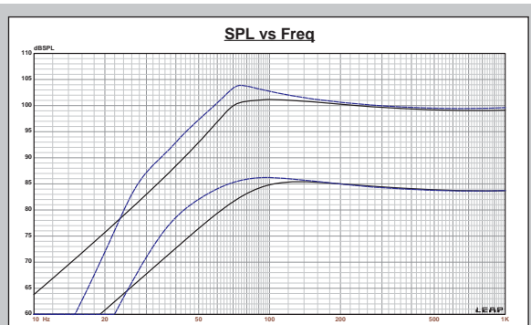
Figure 2: Dayton Audio ES140Ti-8 computer box simulations (black solid = vented at 2.83 V, blue dash = sealed at 2.83 V, black solid = vented at 19.5 V, and blue dash = sealed at 21 V)
