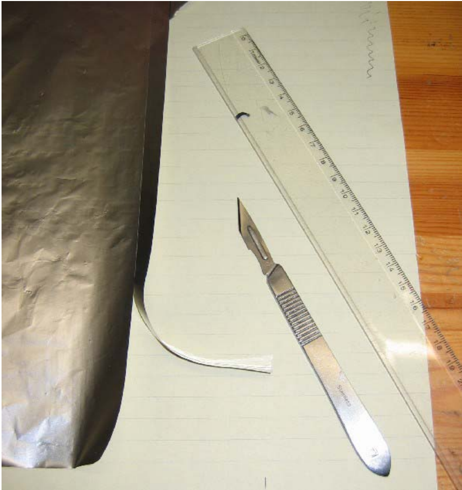
Household aluminium foil, 11 \mu\text{m} thickness. Cut some 8 mm wide strips of aluminium foil with the ruler and the scalpel.
