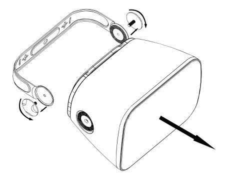
Next install the speaker mounting bracket firmly to the mounting surface using the supplied mounting hardware.
