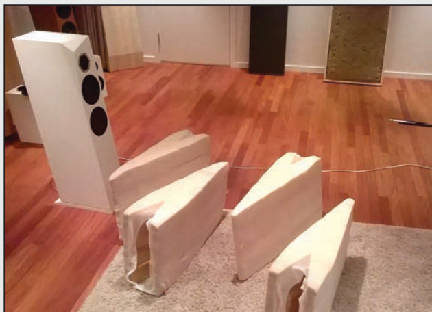
The measurement setup that the designers, Danesian Audio, used for their measurements. Note the asymmetrical shape of the speaker, which are delivered as mirrored pairs.
