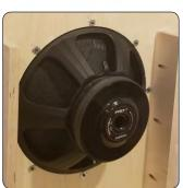
First off is the 12" Bianco-12OB150 woofer with a generous 2.4" voice coil on a fiber glass former, powerful ferrite magnet motor, specified with a high excursion of 18mm, and with a Total Q of 0.63, making it a good choice woofer for open baffle designs. The 12OB150 uses a proprietary cone paper material, combining silk cotton tree and manila pulp, which is then coated with a weatherproof formula.
