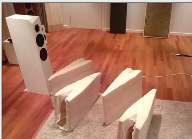
The measurement setup that the designers, Danesian Audio, used for their measurements. Note the asymmetrical shape of the speaker, which are delivered as mirrored pairs.
