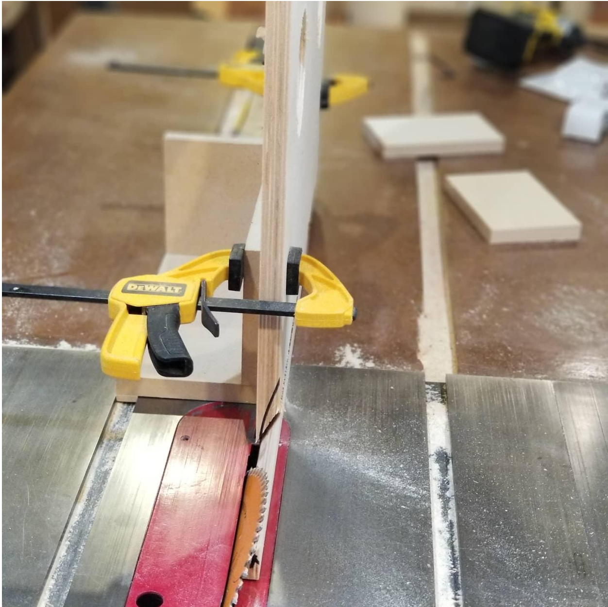
Figure 26 Vertical Miter Cut, jig and clamps to keep me way out of the way of the cut.
