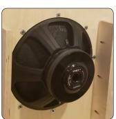
First off is the 12" Bianco-12OB150 woofer with a generous 2.4" voice coil on a fiber glass former, powerful ferrite magnet motor, specified with a high excursion of 18mm, and with a Total Q of 0.63, making it a good choice woofer for open baffle designs. The 12OB150 uses a proprietary cone paper material, combining silk cotton tree and manila pulp, which is then coated with a weatherproof formula.
