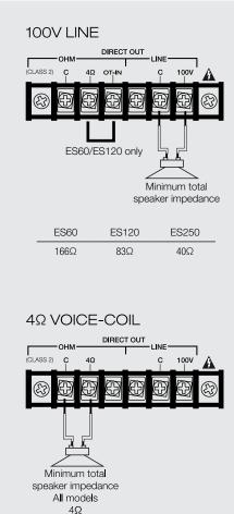
NOTE: Only connect one output – either 100V or  $4\Omega$
