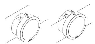
Surface mounted (left) and recessed mounted (right)
