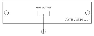
1 HDMI OUTPUT: Connect the HDMI output port to the HDMI input of your display.
