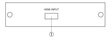
(1) HDMI INPUT: Connect the HDMI input port to the HDMI or DVI output of your source equipment such as DVD player or set-top-box.
