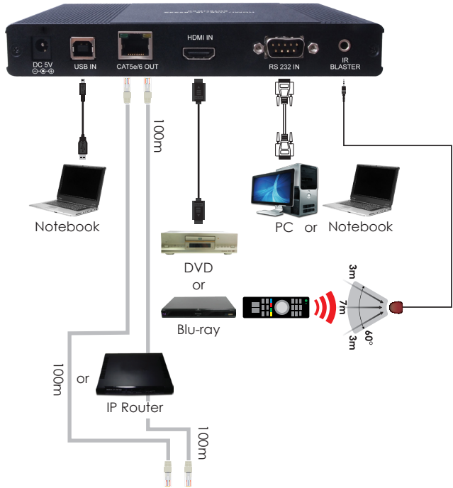
Transmitter's Rear Panel
