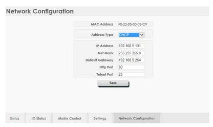
Click on Network Configuration to set the device's IP configuration. Once the changes are saved the system will reset the IP address on device automatically and user will need to re-enter the IP address to continue the WebGUI function.
