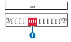
EDID: The EDID dipswitch block provides a way to select the EDID to use with the connected source. By using a combination of on and off settings for the dipswitches, there are a total of 16 possible EDID selections across 3 different operation modes.
