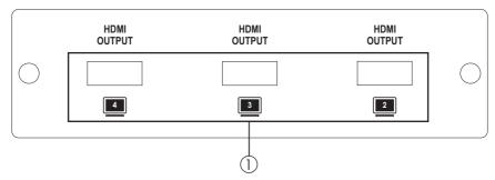
① HDMI OUTPUT 2/3/4: Connect each of the output ports to an HDMI display. When more than one output source is connected, an identical video signal will be shown on the connected displays.
