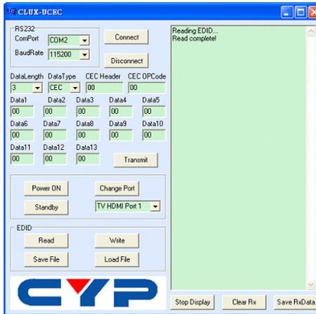
When the EDID has been read successfully, the communications log window will show "Read complete". Click on the Save File button to save the EDID in the user's desire.
