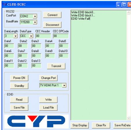
If the communications log window shows "EDID Write Fail", check the connection to the device and make sure it is well connected and powered up and also check the EDID file is correct then click on the "Write" button to try again.
