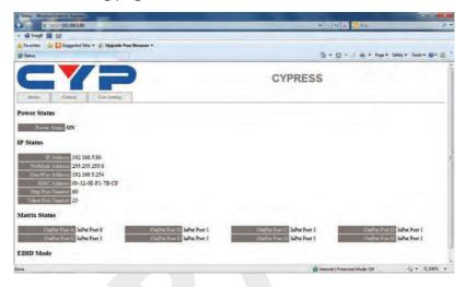
Click on the 'Control' tab to control power, input/output ports, EDID and reset mode.
