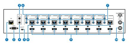
**1** LAN: Connect to an active network for LAN serving and Telnet and Web GUI control (refer to Sections 6.8 and 6.9).
