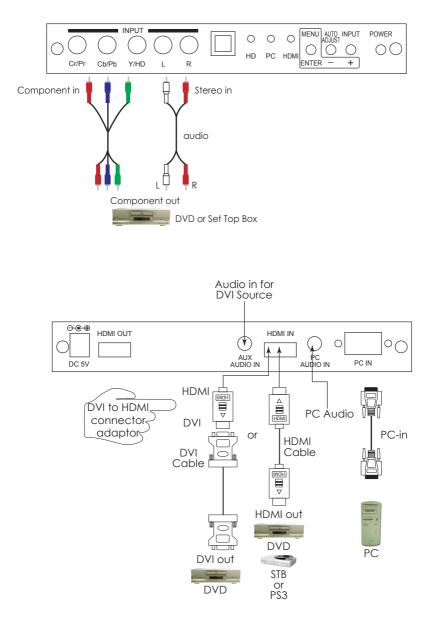
The CP-255H accepts component, PC and HDMI inputs with audio on each. The formats supported by these inputs are as follows:
