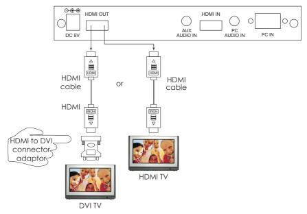
The CP-255H can output a variety of PC, SD and HD resolutions in HDMI digital format.
