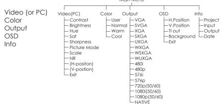
Use +, - button to move hightlight bar to your desired parameter, then press MENU/ENTER to enter into sub-menu of your selected parameter.
