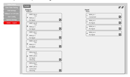
To begin assigning a new video route, please click the button of the HDBaseT output you wish to send video to (e.g. "HDBT\_Out A") and then click on the button of the preferred HDMI input port (e.g. "HDMI\_In 1"). If desired, you may select more than one output prior to selecting the input. As you select each button they will change their color to orange. The new route will become active immediately and the routing information displayed on the buttons will change accordingly.
