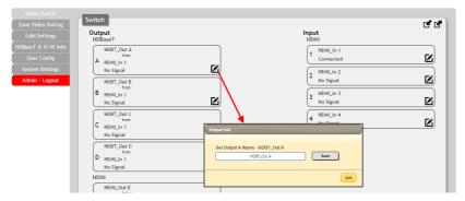
All inputs and outputs can be renamed as required. To rename the HDBaseT output ports and HDMI input ports please click the "edit" icon (🗹). Click the "Save" button to confirm the change.
