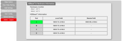
This page provides information concerning the temperature inside the matrix near critical components (areas 1 & 2) and the HDBaseT firmware versions used in the matrix and in connected receivers.
