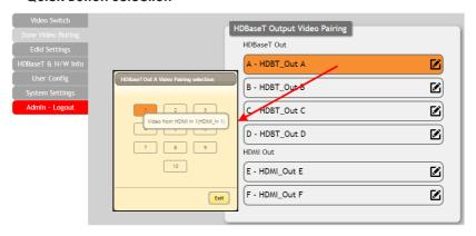
To activate a video pairing from the WebGUI, please select the HDBaseT output port to launch the selection window. The numbers  $1\sim10$  correspond to the keys on remote control unit.
