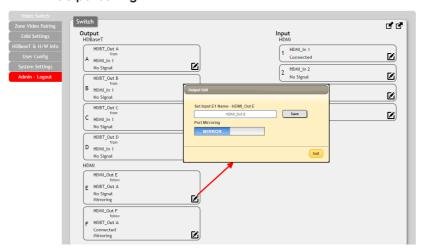
The two HDMI outputs (port E & port F) allow support for the maximum HDMI timing up to 6G (4096×2160@60Hz) and can be used for normal source routing (listed as "Independent" within the WebGUI) and mirroring (listed as "Mirror" within the WebGUI) for local monitoring purposes or zone monitoring (e.g. The HDBaseT output connects to a TV in a remote zone the local HDMI connection goes into an AVR ).
