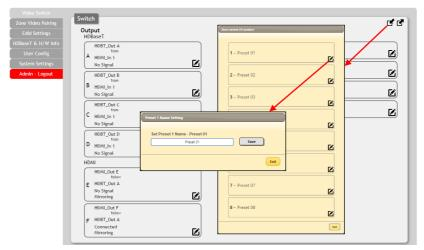
This matrix can store up to eight video and audio routing presets. Presets can be utilized to store multiple different routing states in advance for rapid, hassle-free, recall.
