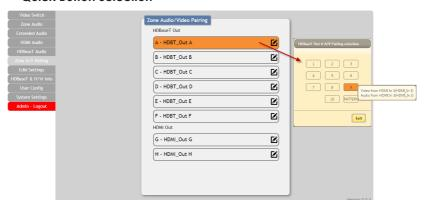
Please select the HDBaseT output port first and then click the "edit" icon (🗹) to launch the window for further adjustments. The numbers 1~10 and "pattern" correspond to the keys on remote control unit.
