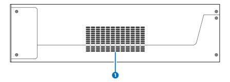
1 FAN VENT: These are air ventilation areas. DO NOT block these areas or cover them with any objects. Please allow adequate space around the unit for air circulation.
