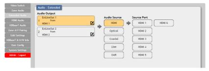
Click the buttons from left to right to choose each output's source. Once the new source has been selected, the change will happen immediately. Audio source options include HDMI, Optical, Coaxial, Line, and OAR.
