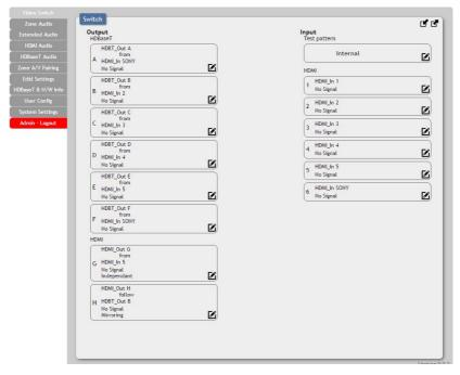
To begin assigning a new video route, please click the button of the HDBaseT output you wish to send video to (e.g. "HDBT\_Out A") and then click on the button of the preferred HDMI input port (e.g. "HDMI\_In 1"). If desired, you may select more than one output prior to selecting the input. As you select each button they will change their color to orange. The new route will become active immediately and the routing information displayed on the buttons will change accordingly.
