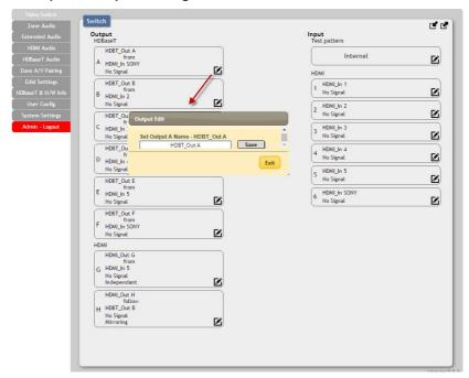
All inputs and outputs can be renamed as required. To rename the HDBaseT output ports and HDMI input ports please click the "edit" icon (2). Click the "Save" button to confirm the change.
