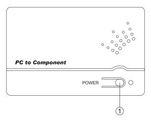
1 Power switch and LED Indicator: When power is turned on the LED will illuminate in green color. When press power switch once to turn the system in standby mode and the LED will illuminate in red color. Note: The factory setting is in power on mode.
