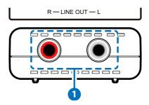
**1 R/L LINE OUT:** Connect the L/R analog audio output to the input of your AV Receiver or audio system.
