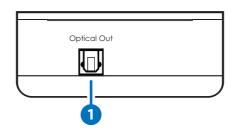
**Optical Out:** Connect to the Optical input of an AV Receiver or active speakers.
