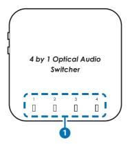
1 Input LED 1~4: The blue LED will illuminate to indicate the selected source.
