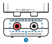
**1 LINE OUT:** Connect the R/L OUT to an analog stereo (R/L) amplifier or active speakers for audio output.
