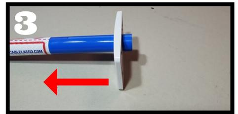
Insert tool into brick wall until face plate meets wall
