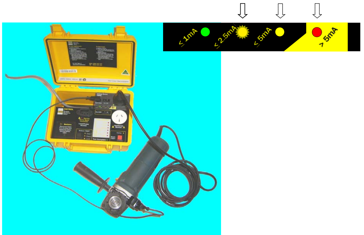
Figure 4.6-2 Class II Appliance Fail.
