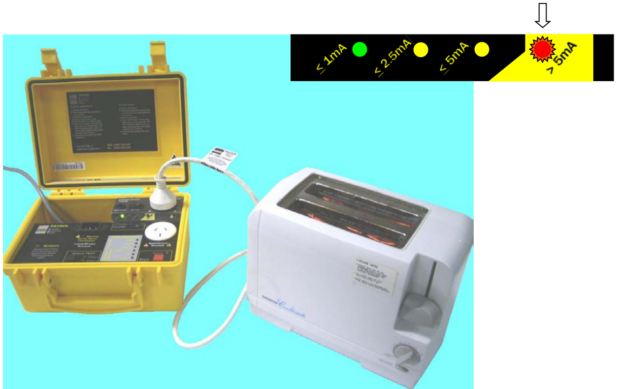
Figure 4.6-1 Class I Appliance Fail.
